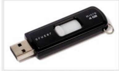
A USB flash drive is physically much smaller than a floppy disk, but has a capacity thousands of times larger.
